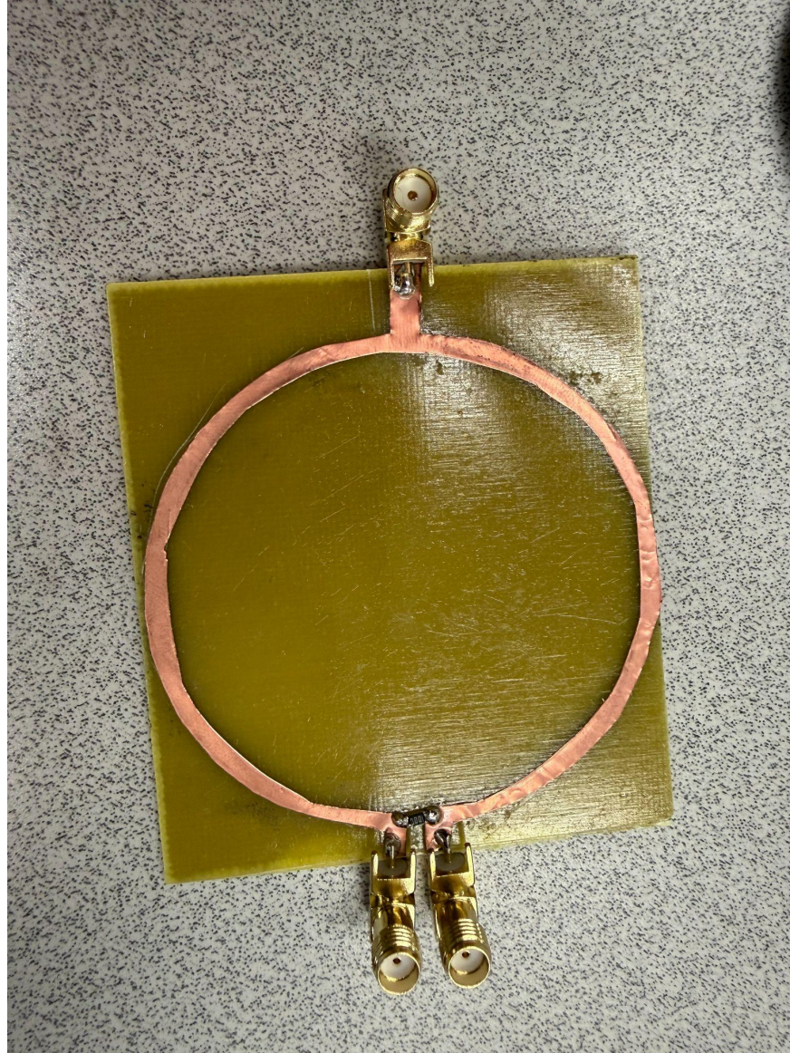
Figure 4. Fabricated Wilkinson power divider using copper tape and SMA connectors
