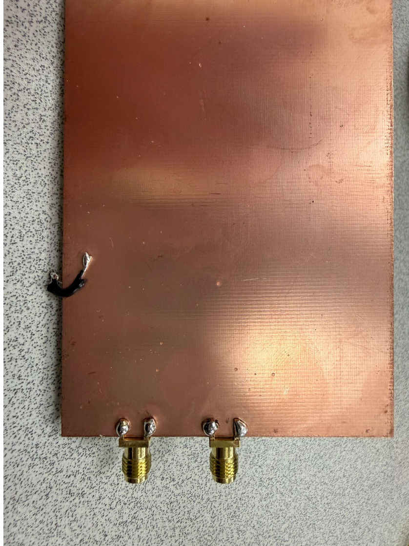
Figure 11. Copper ground plane used on the underside of the FR4 amplifier board.
