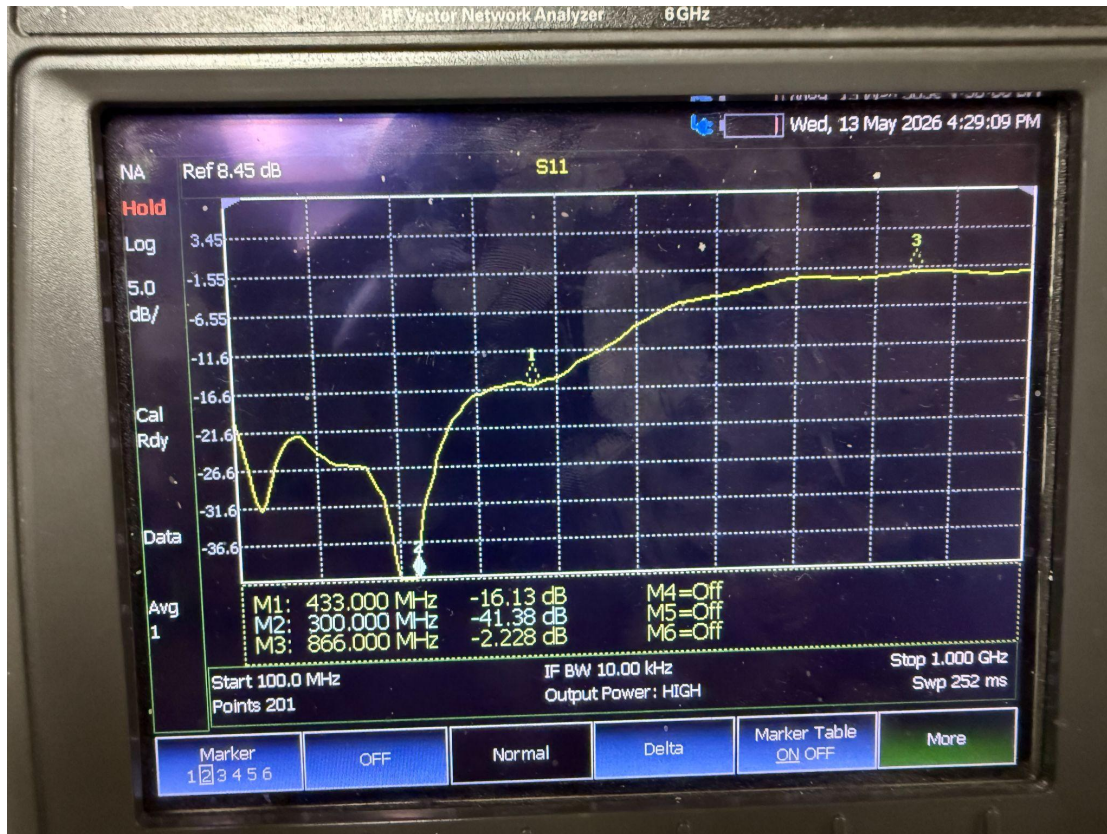
Figure 7. Measured S11 response of the fabricated low pass filter using the Vector Network Analyzer.
