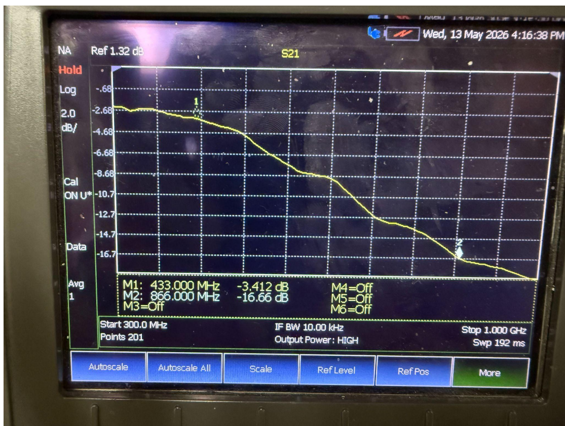
Figure 6. Measured S21 response of the fabricated low pass filter using the Vector Network Analyzer.
