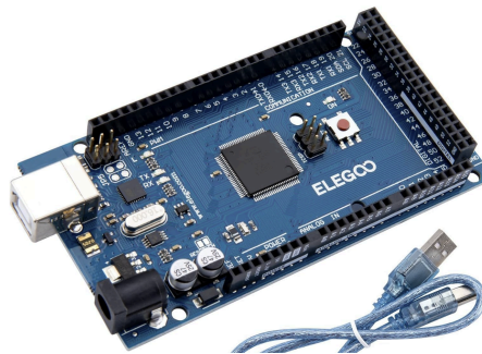
Figure 5: ELEGOO MEGA R3 Board ATmega2560
