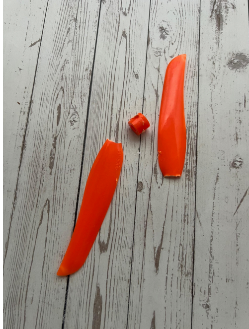
Figure 11: Broken Propeller from incorrect PID values
